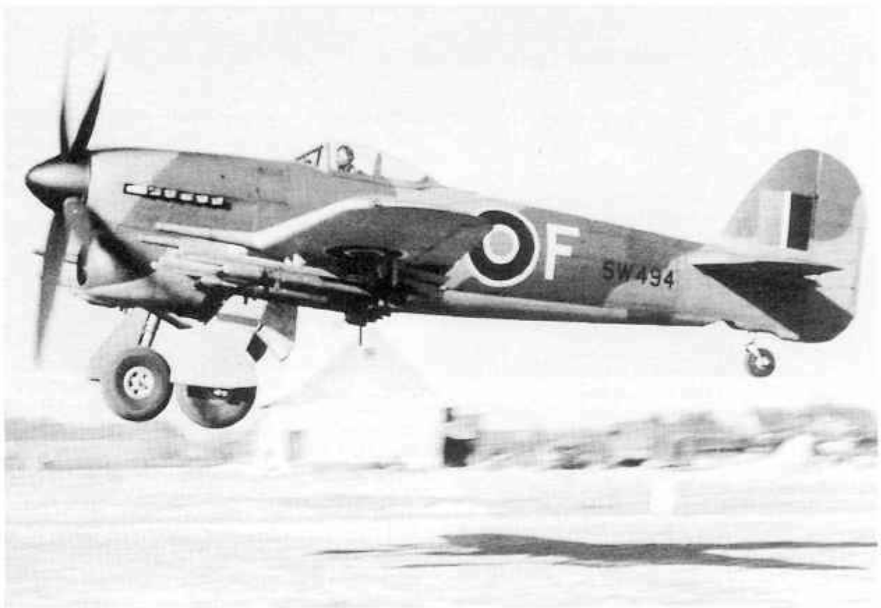
A Typhoon takes off on a mission carrying its potent load of eight 3-inch rockets.
